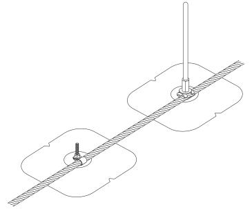
**ASCE 7-16** code requires all rooftop equipment to be bolted, welded, or otherwise positively fastened without consideration of frictional resistance.
