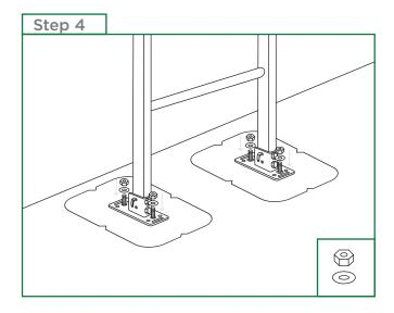
Secure the base of the ladder over the U-Anchor bolts using the provided Stainless Steel Flat Washers and Flange Nuts.
