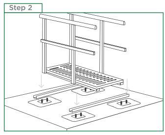
Install the pass-through bridge first. Place the base channel over the U-Anchor bolts perpendicular to the placement of the final location of the pass-through bridge secure the bridge brackets to the channel using the provided channel nuts/bolts.
