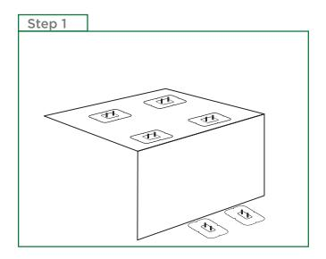
Align the U-Anchors in accordance with the ladder and pass-through bridge design. Install the U-Anchor as per instructions provided by Anchor Products and in compliance with the roofing manufacturer requirements. Make sure to follow any applicable pre-installation and post-installation requirements according to the engineered design.
