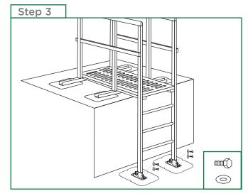
Position the ladder over the lower roof U-Anchor bolts and lift into position (make sure to not damage the roof surface) and secure the top bracket of the ladder to the pass-through bridge. Use the provided hardware.
